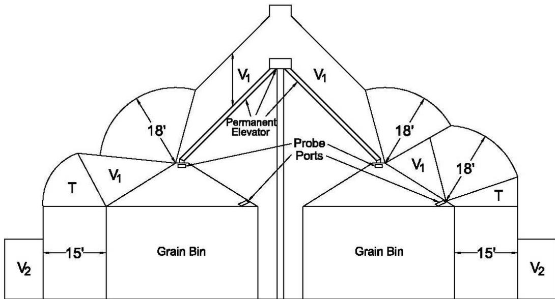
$V_1$  = Vertical clearance above a building required by Rule 234C (Table 234-1)
